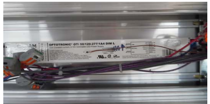
Indirect Driver Thermocouple Location
