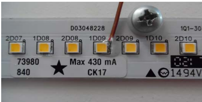
Indirect LED Thermocouple Location
