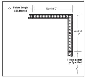
Lighted Horizontal Corner (High, Medium or Custom Output LED) Consult Factory for exact luminaire placement.
