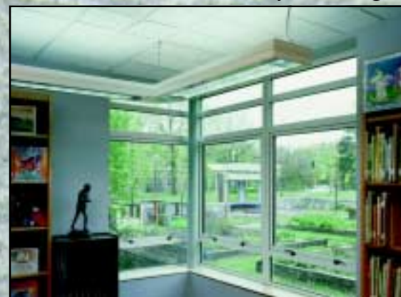
The Trilinea system's 90-degree cast corners provide seamless connections between fixtures. The Trilinea obround is also available with 'T' and 'X' connectors for greater pattern flexibility.
